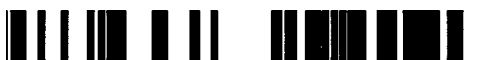
FIG. 11. Realization of an overlapping-rod system: The system size is 1000 pixels. The rod length is 10 pixels and the area fraction of phase 1, \phi_1=0.5 .
