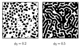
Figure 6. Construction of digitized two-dimensional realizations (400 pixels × 400 pixels) that computatively correspond to the target function given by eq 34 for  $\phi_2 = 0.2$  and 0.5.<sup>3,9</sup> Here, a = 32 pixels and  $q = 8\pi/a$ . We now know that this function is not exactly realizable, because even though the construction technique matched eq 34 for almost all r, it could not yield the necessary convex behavior in the vicinity of the origin.
