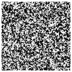
Figure 3. Construction of a digitized two-dimensional realization of a "Debye" random medium (400 pixels × 400 pixels).<sup>3,7</sup> Here, the volume fractions are  $\phi_1 = \phi_2 = 0.5$  and the correlation length is a = 2 pixels.
