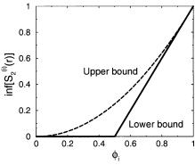
**Figure 1.** Graphs of the upper bound (dashed curve) and lower bound (solid lines) of expression 20 on the infimum of  $S_2^{(i)}(r)$  for a statistically homogeneous medium.
