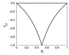
Figure 2. Graphical depiction of the bounds described by expression 25 on the infimum  $(f_{inf})$  for volume-fraction-independent f(r). The quantity  $f_{inf}$ must lie within the region delineated by the heavy solid lines.
