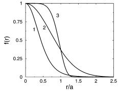
Figure 4. Examples of scaled autocovariance functions that cannot correspond to statistically homogeneous and isotropic two-phase random media:  $f(r) = 1/(1 + r^2)^4$  for  $d \le 5$  (curve 1);  $f(r) = \exp(-r^2)$  for any d(curve 2); and  $f(r) = \exp(-r^6)$  for any d (curve 3).
