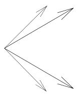
Fig. 3. A finite deformation of the bitriangular lattice. A large deformation of the unit cell of the bitriangular lattice is shown using the lattice vectors. The original vectors are shown with a solid line, while the final ones are shown with a dashed line. During this deformation, the unit cell shrinks and becomes a square. We ensure that the lattice does not rotate so that it is possible to achieve this deformation by integrating a symmetric (time-dependent) strain rate.
