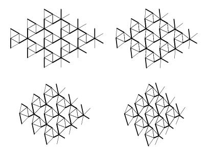
Fig. 4. Achieving the deformation from Fig. 3. This sequence of time frames (as in Fig. 2) shows how one can achieve a global uniform deformation of the bitriangular structure during which the unit cell shrinks and becomes square by only actuating the three active arcs. Notice that the inactive arcs do not change length and therefore this actuation does not store any elastic energy. The mathematics used to produce this illustration is given in the ODE system of Eqs. (14)–(16).
