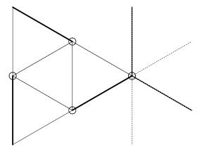
Fig. 1. The unit cell of the bitriangular framework. The 4 joints in the unit cell are shown as circles, while the 9 bars in the unit cell are shown with a solid line. The three active arcs are shown with thicker lines, and the periodic images of the arcs with non-zero  $\mathbf{n}_c$  are also shown with dashed lines.
